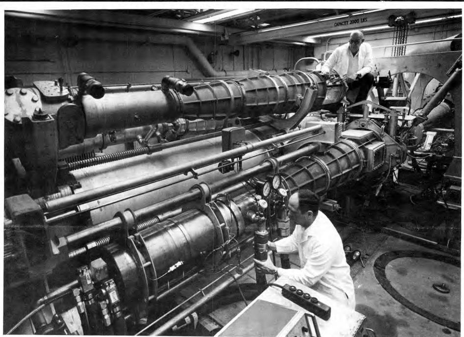
HYPERSONIC WIND TUNNEL facility in Bldg. 865 was scene recently of the first successful Mach 14 run. Don MacKenzie adjusts cooling hoses to the throat section while
